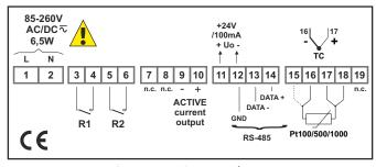
85-260V +24V /100mA 6,5W + Uo -N 2 5 6 7 8 9 10 11 12 13 14 15 16 17 18 1 3 4 n.c. n.c. DATA + OC1 OC2 PASSIVE isolated GND current Pt100/500/1000 RS-485 CE output
